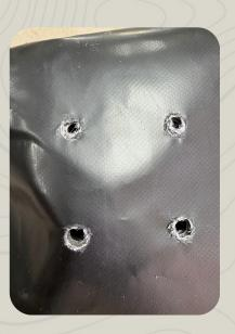
**4.** Insert M8 bolts on the existing four (4) holes of the awning hinge and through the mounting bracket.
