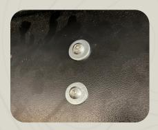
**5.** Insert two (2) button head bolts with M8 washers in the two existing holes on the awning pan and the mounting brackets. Fasten using a 13 spanner and 5 Allen key.
